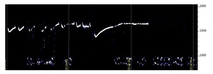
The "height" of this chirp is 272Hz and it takes 12.6 seconds to cover that frequency range. This is therefore a significant improvement over 510Hz in 4.3 seconds. But it is not exactly a massive change!
