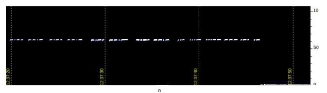
In yet another attempt to analyze it a different way, I tried making an Audacity recording. Then I selected a few milliseconds of the recording and ran the FFT tool to identify the frequency. I repeated this at various times after the start of the key-down and tried to plot it in a spreadsheet. Below is a screenshot from my computer. It was quite hard to measure consistent results with this method, and very time consuming, so I quit.
