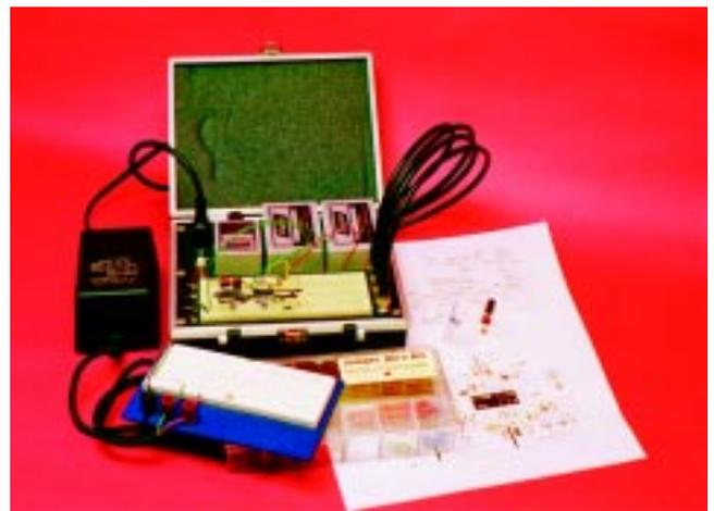
Figure 6. The circuit of Figure 5 was constructed from two integrated circuits (with one amplifier left over!) on a shop-built prototyping rig. The rig contains precision power supplies and a convenient way to interface BNC connectors with the circuit. Commercial development boards, such as that shown, can also be used to build small circuits. Planning the component placement before patching is always a good idea . . . note the pictorial layout.
