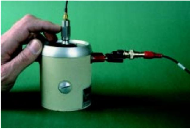
Figure 8. 'Pluck' testing an LDS model V-203 shaker. The finger depresses the table against its limit stop, then releases it abruptly. The voltage generated by the shaker coil is measured with a high impedance instrument. Comparative spectral measurements made between a bare table and one loaded with a known mass permit identifying the suspension parameters.
