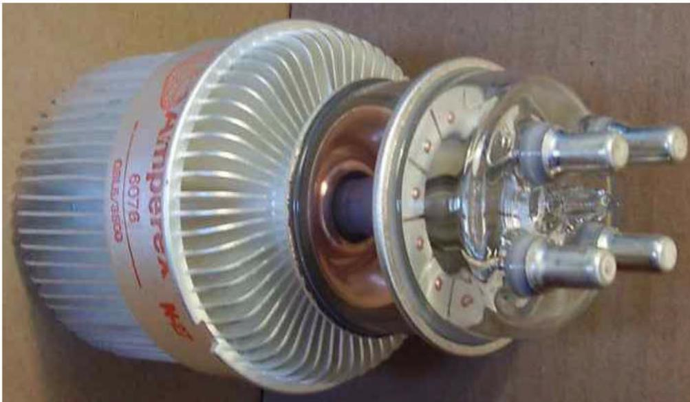
6076 is a forced air cooled transmitting tetrode. 3.5KW, 220MHz. Intended for FM-TV transmitters.
