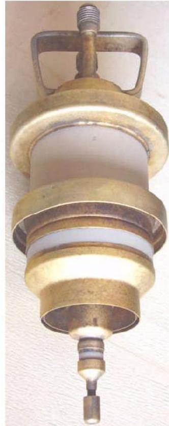
Two transmitting tubes from General Electric. GL-434-A was used in early radar applications. The coaxial tetrode GL-6019 delivers 1KW output at 900MHz. Water cooled, it was intended for UHF TV transmitters.
