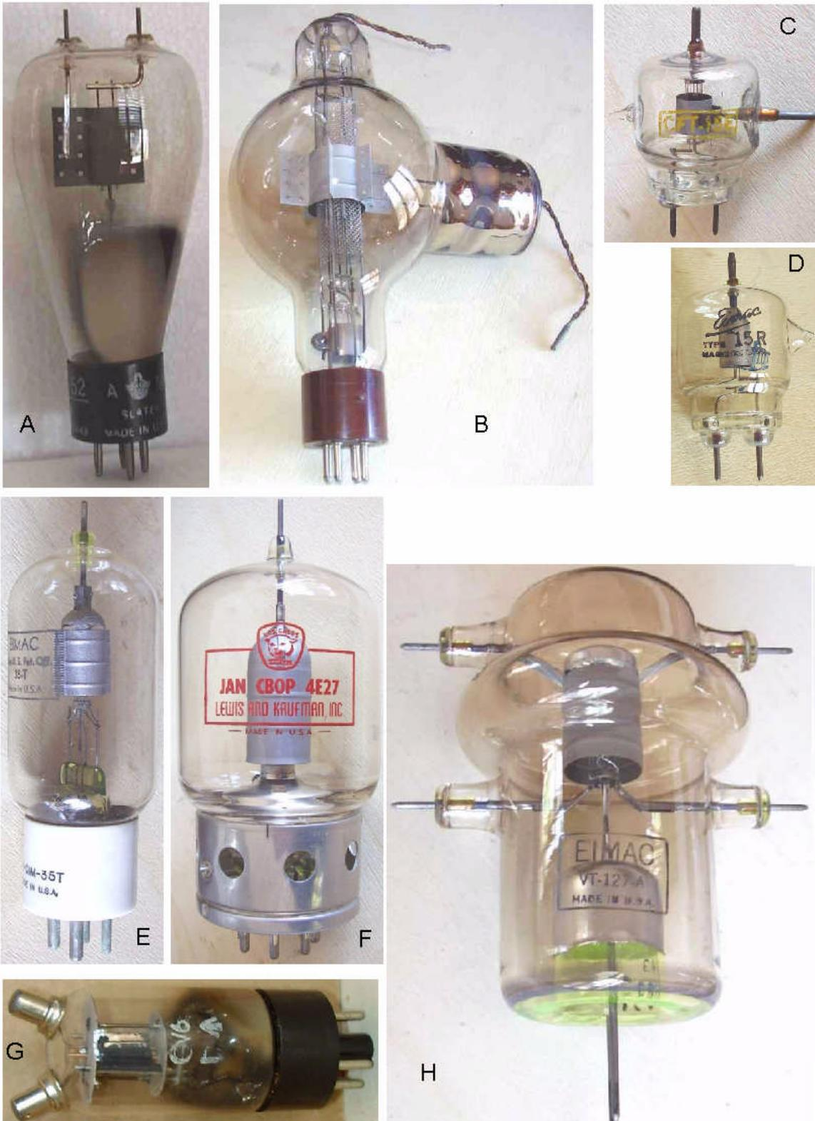
From early 930s to the eve of WWII there were continuous improvements in low power VHF transmitting tubes, intended for FM, early TV systems, radio relays and radar equipment. Solutions included short connections to grid and anode, baseless connections, special materials, as tantalum, for electrodes and hard glass bodies.
