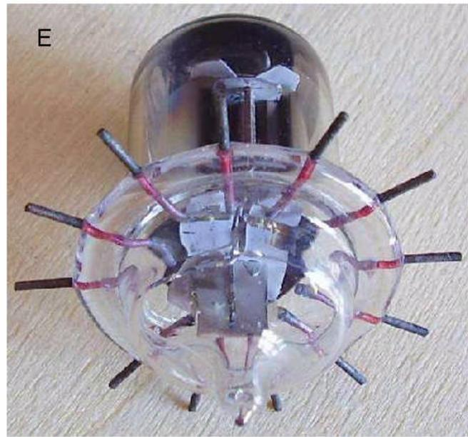
Acorn tubes were introduced around the mid 930s to reduce parasitic parameters, inductance and capacitance, of the connections. Pins went out radially from the glass press around the body and sometimes from the top and from the bottom. When the miniature 7 pin bulbs appeared, the small electrode structures of the acorn tubes were readily moved to the new envelope, without appreciable decrease in high frequency performances.
