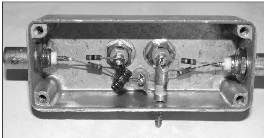
Fig 8—Inside view of crystal measuring test fixture.
