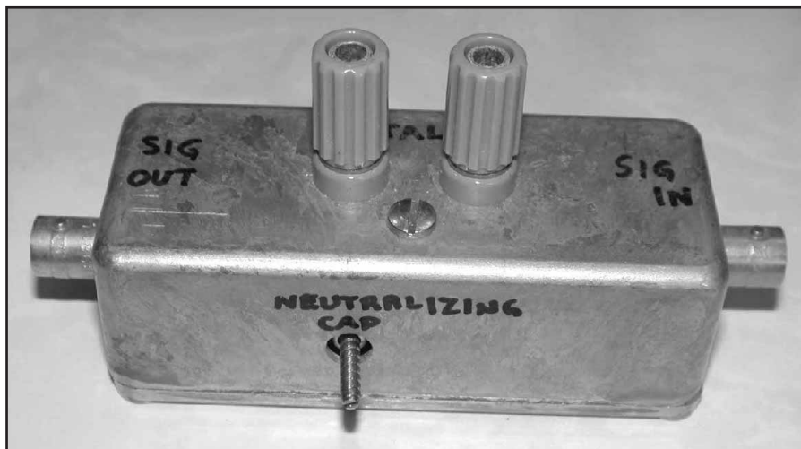
Fig 7—Outside view of crystal measuring test fixture.
